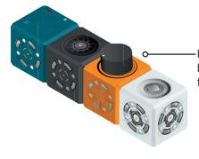
It is important to place the Threshold between the SENSE and ACT Cubelet for it to function as intended.
