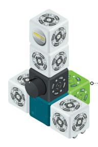
• The Passive Cubelet helps balance this robot construction. Challenge your students to use the Design Thinking Process to design a robot that doesn't tip over.
