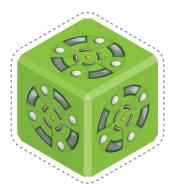
PASSIVE Transmits power and data like a wire, and can extend and stabilize robots.
