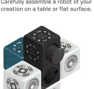
Here is an example of a complete robot that drives and shines a flashlight! Do you see that it has a Battery for power, at least one Sense Cubelet, and at least one Action Cubelet?
